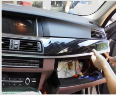
1. Pry up AC vent panel.
