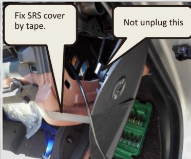
10. Put USB cable into container, bring cable passing through right SRS cover, Note: Fix SRS cover by tape, not unplug flat cable, or else SRS fault code will show up.
