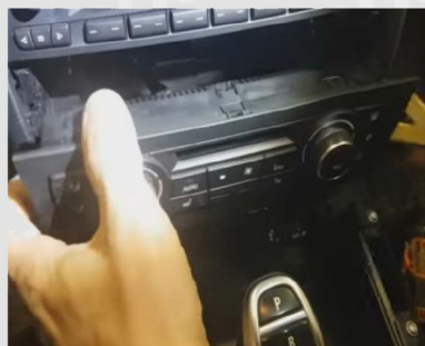
7. Use crowbar to prize up A/C panel and take off flat cable.
