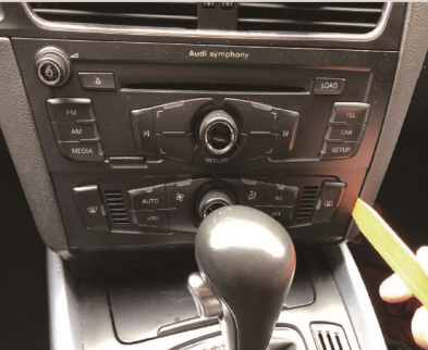
5. Remove the original A/C control panel off.
