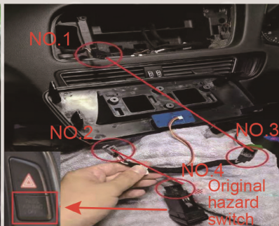
15. Some car has an airbag indicator on the emergency light button, android screen has no such button, you can connect it, and leave it inside car.
