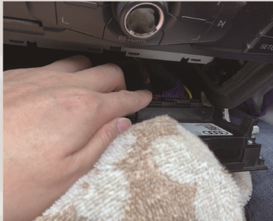
6. Remove the data cable off A/C control panel.
