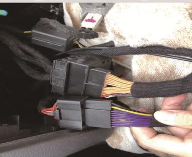
9. Connect power cable to A/C wire plug.
