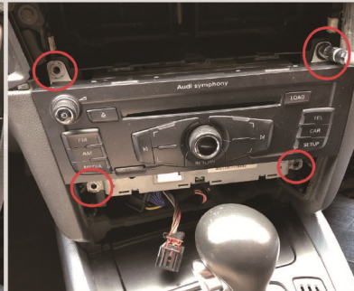
8. Take 4 fixing screws off car CD.
