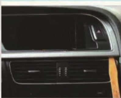
2. Pry out the panel around original screen, remove the emergency light data cables.
