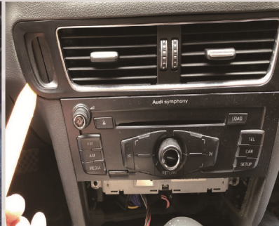
7. Dismantle A/C wind panel, take off data cable.
