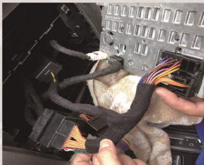
10. Connect the male plug of power cable to CD headunit.
