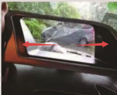
14. Dismantle the black frame off and put back silver panel.
